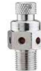
Air Vents 1/4" CHROME PLATED AUTO AIR VENT • Brass with BSP male parallel thread • 10bar max
