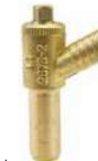
Type A Draincock TYPE A DRAINCOCK IN VARIOUS SIZES • Sturdy brass construction • Supplied with seal inside body, this keeps the product watertight when not in use • No need for a specific key to tighten • Water flow can be easily adjusted by use of a spanner
